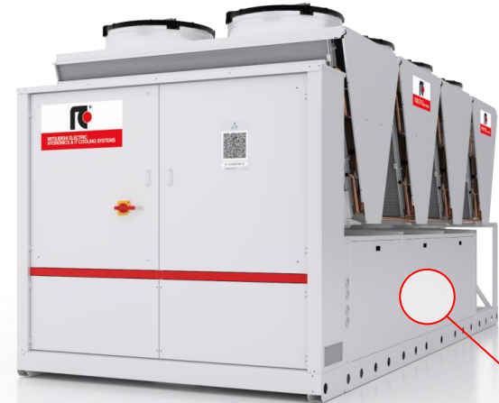
The compressors and the refrigerant circuits are below the V-block coils. Compressor enclosures are provided upon selection of opt. 2312 Acoustical enclosure or opt. 2282 NR kit
